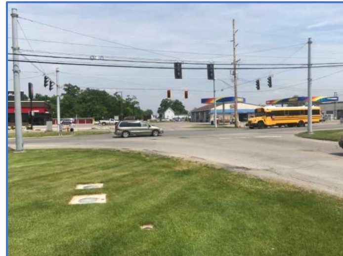
Photo 24: Monitoring wells throughout property. Potential Brownfield/Remediation ongoing.
